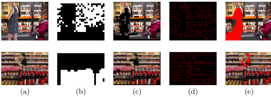
Figure 3: Intermediate results after each step on synthetic examples (a) Input spliced image (b) Result of PSF grouping (all white pixels belong to single depth layer) (c) Patch classification after comparing the blur kernels through correlation (d) Texture based segmentation of the input image using [22] (e) Final result showing localized spliced region in red
